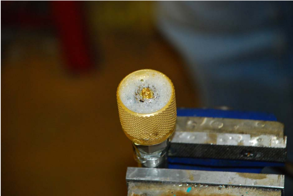
Photo 1 Coupling showing a leak.
